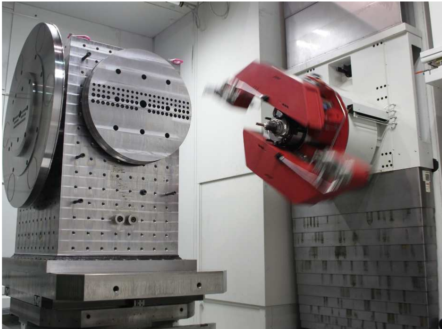
Planetary TurnMill Device (PTM): milling, drilling, lathing with one support
