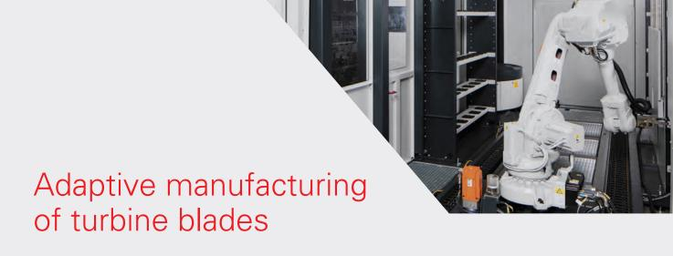
Starrag has developed a flexible manufacturing system with four machining centres for the safe, customer-specific series production of turbine blades, embodying the core concepts of Industry 4.0.
