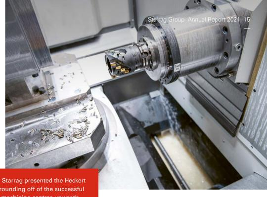
Virtually highly dynamic: Starrag presented the Heckert H65 via video stream, a rounding off of the successful Heckert 4-axis horizontal machining centres upwards. With its compact design, this new addition can process workpieces weighing up to 1.5 tons.
